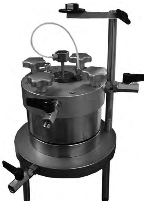
Figure 17.7 Hydraulic consolidation (Rowe & Barden) cell for test specimens of 50, 63.5, 70, 76.2 and 100 mm diameter'
